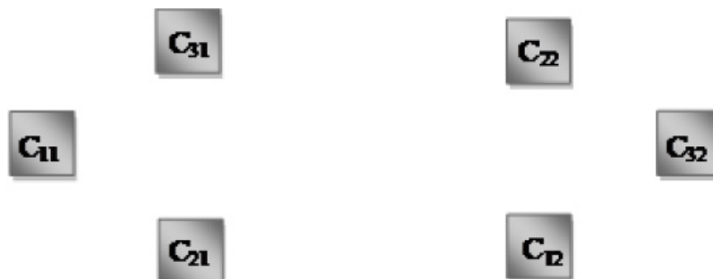
Figure 2: Schematic of the two triangular arrangements of the three-square cylinders considered in this study.
