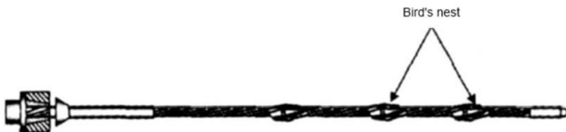
Figure 8: Structural sketch of bird's nest anchor cable.
